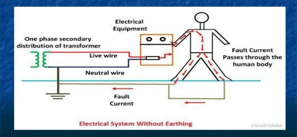
When the fault occurs the fault current from the equipment flows through the earthing system to the earth and thereby protect the equipment from the fault current. At the time of the fault, the earth mat conductors rise to the voltage which is equal to the resistance of the earth mat multiplied by a ground fault.
