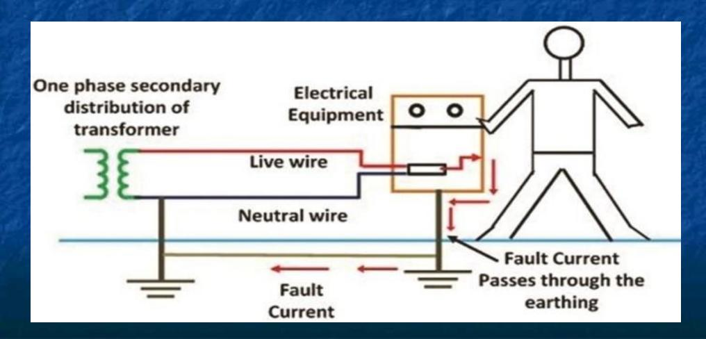
The contacting assembly is called earthing. The metallic conductors connecting the parts of the installation with the earthing are called electrical connection. The earthing and the earthing connection together called the earthing system.
